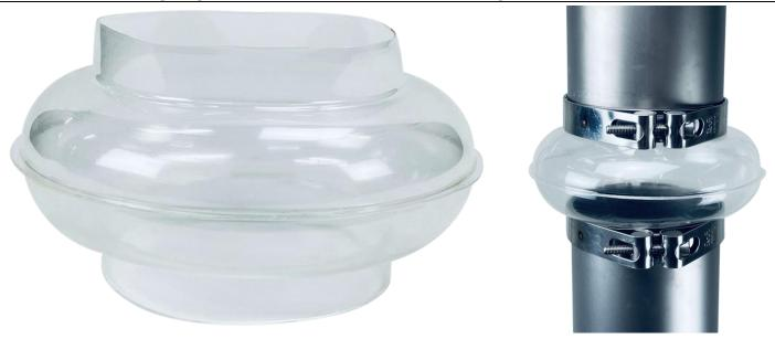
The classical Spherical Bellow shape has been designed to transfer minimal influence such as vibration or movement from the feeding or receiving equipment to the weighing or dosing equipment. This design is excells in compensating large axial movements, such as compression or exstension. The axial compression movement allows for easy 10 to 20mm of travel, or an absolute maximum of 50mm.
