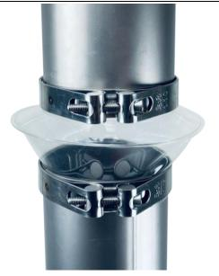
The asymmetrical conical shape has been designed to prevent any powder from sticking to the lower half of the bellow. At a 60° Angle its slope is steep enough for powder not to collect inside the bellow. The upper cone allows a 10mm axial compression movement.
